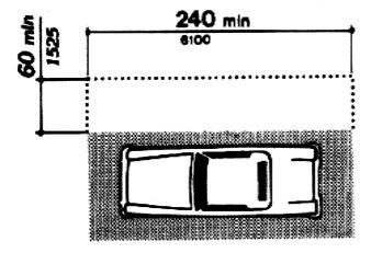
**Parking Spaces.** Accessible parking spaces shall be at least 96 inches wide. Parking access aisles shall be part of an accessible route to the building or facility entrance. Parking spaces and access aisles shall be level with surface slopes not exceeding 1:50 (2%) in all directions.
